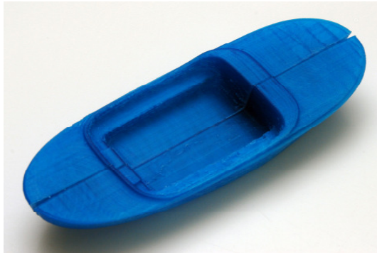
Fig.2: Ultimaker print of motor launch, printed in two parts (SB and PS)
